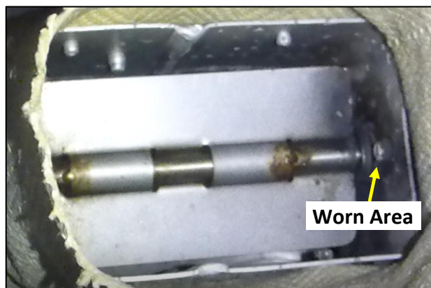
Photo No. 2: Carburettor heat flap housing worn in area of flap spindle
